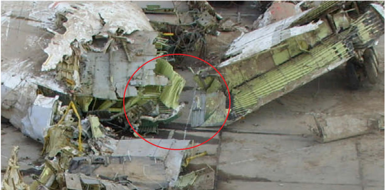
Fig. 16. The plane wreckage shows missing parts in the area of the central fuel tanks.
